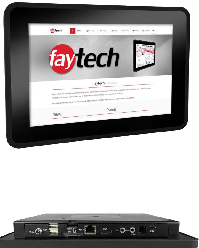
faytech's Embedded Touch PCs have a pre-installed Android 6 operating system and are equipped with W-LAN module. The device has an IP65 water- and dust proof front panel with capacitive 10-finger multitouch. All the PCs have VESA 75 or VESA 100 screw patterns on the back, while the 13.3" to 27" come with their own desktop stand included.
