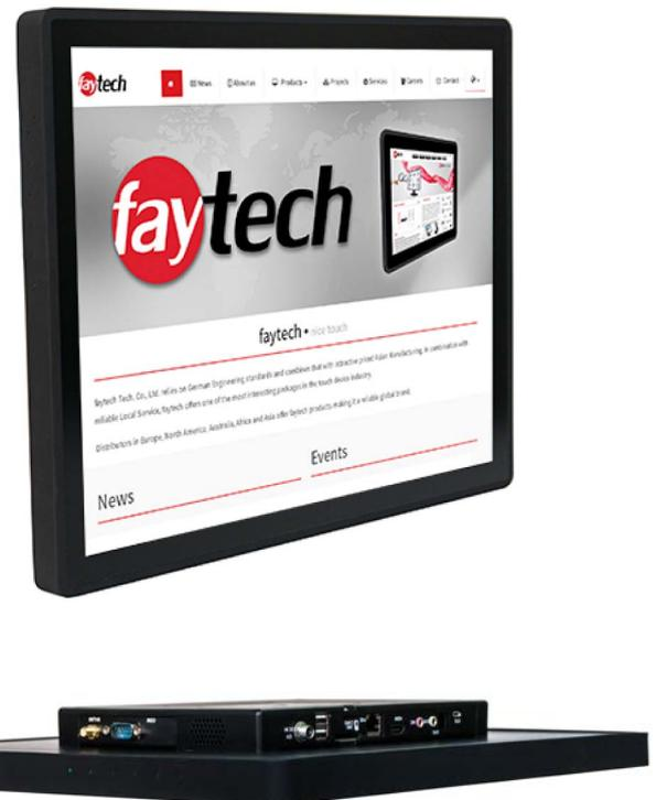
faytech's Embedded Touch PCs have a pre-installed Android 6.0 operating system and are equipped with W-LAN module. The device has IP65 water- and dust proof front panels and capacitive 10-finger multitouch. All the PCs have VESA 75 or VESA 100 screw patterns on the back, while the 13.3" to 21.5" come with their own desktop stand included.
